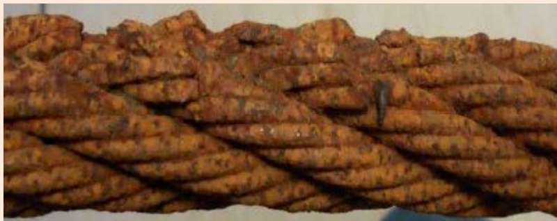
Wire rope fibre core with extensive corrosion, pitting, and broken strands visible on the exterior.
